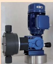
The electric pump DTK is a model of volumetric pump with direct diaphragm. The membrane is mechanically moved by a movement of reciprocation driven by an electric motor.
